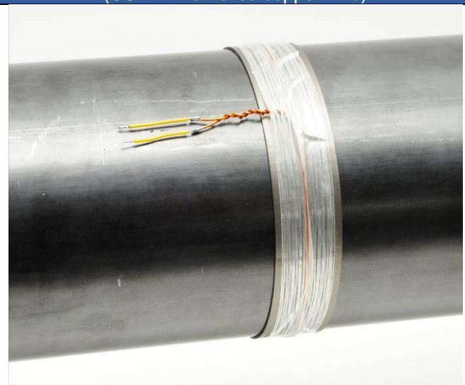
Extend the CUL wire flexible 0.14-0.25mm wire (to decouple the inflexible 1mm wire!, at 0.63 not necessary)
