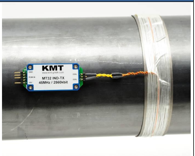
Twisted also the flexible wire and solder it on the MTP-IND-Tx (isolate all solder points with shrink tubing)
