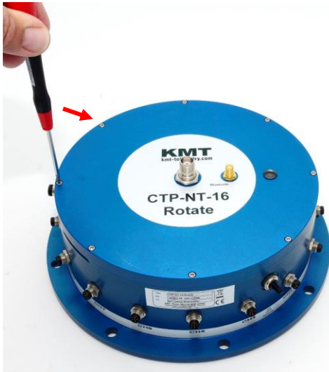
1. Open 8x hexagon screw (2.5mm) with 2mm screw driver
