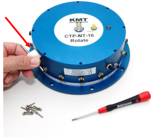
2. Use cover lifter to open the cover carefully
