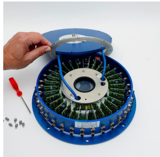
4. Move the modules holder ring to the rear (it is not necessary to disconnect the antenna blue cables)
