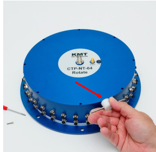
2. Use cover lifter to open the cover carefully
