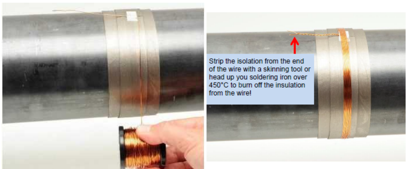
Make power coil with 3-18 windings for 1000-20 mm diameter (see diagram) and twisted the end of wire. Use 0.63...1.00 mm (1.00 mm for diameter of 100-1000 mm) CUL wire (Enameled copper wire)
