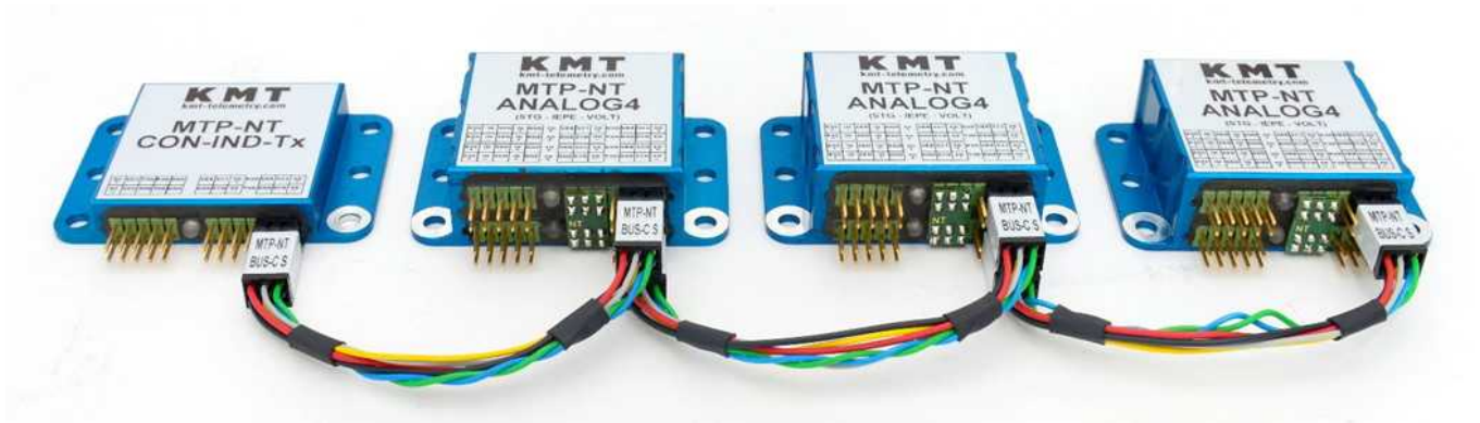
connection scheme 4 channel version
