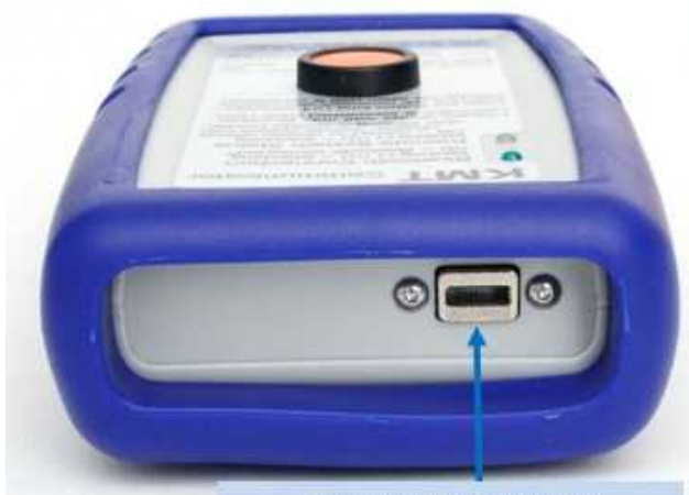
Micro-AB USB Receptacle for powering and communication to PC
